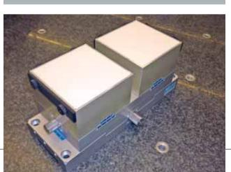
Rotary vacuum clamping chuck with  $\ensuremath{\mbox{\sc porous}}$  clamping surface
