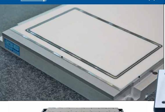
Vacuum clamping system for laser application. Detail shows both clamping areas and cutting channels.
