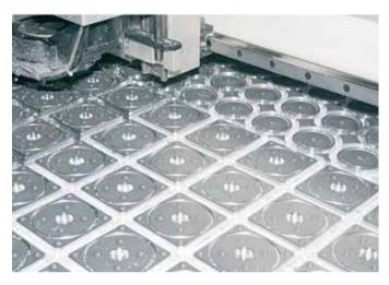
Machining of aluminum sheets of greater thickness
