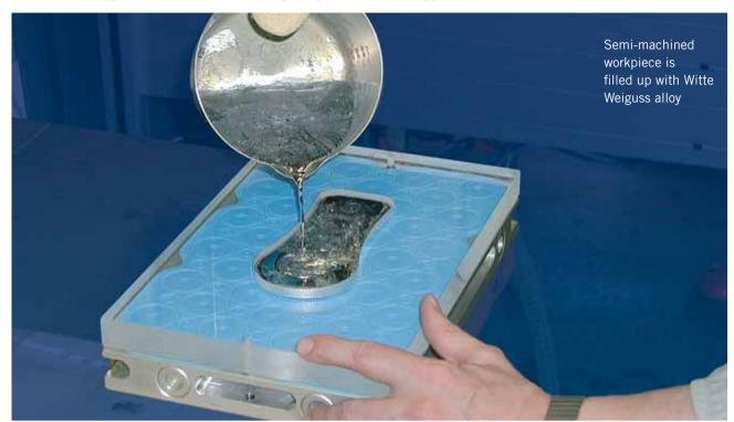
**Witte Weiguss** mould clamping technology is suitable for manufacturing workpieces, which cannot be clamped conventionally because support surfaces are lacking.
