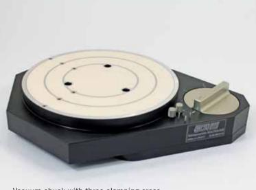
Vacuum chuck with three clamping areas and lifting pins for **manually** controlled process
