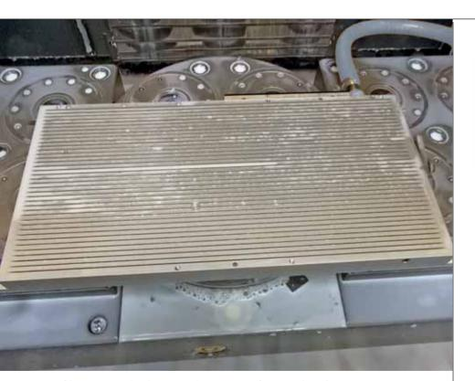
Slot vacuum chuck mounted on a zero reference clamping system
