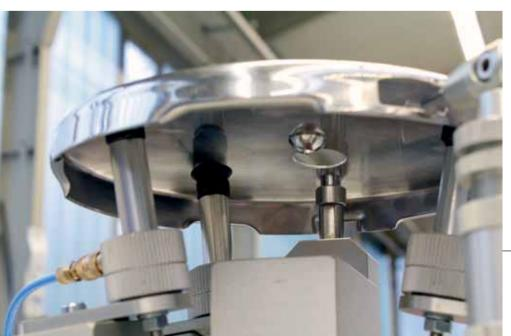
Fast clamping for complex shaped parts
