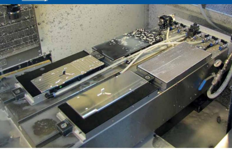
4 slot chucks on a machine used for manufacturing aluminium carriers. Machining of inner and outer contours is done in one process thanks to rubber adapter mats.
