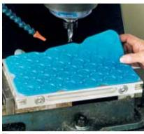
The lugs underneath the mat guarantee fast and accurate positioning of the VAC-MAT™ on the special modular vacuum chuck
