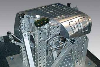
3D vacuum fixture for fixation of pre-formed aluminium parts. Complex contours are milled and cutouts held securely while under the influence of vacuum downforce.
